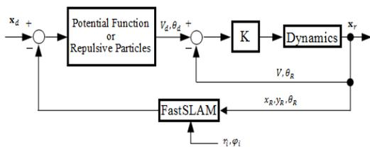
Figure 6. Block diagram of proposed control system.
