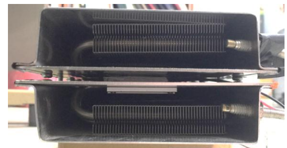
Figure 3. Cross sectional representation of heat exchanger device
