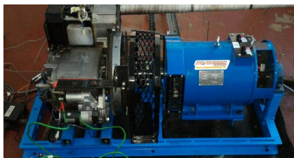
Figure 2. Engine and dynamometer assembly
