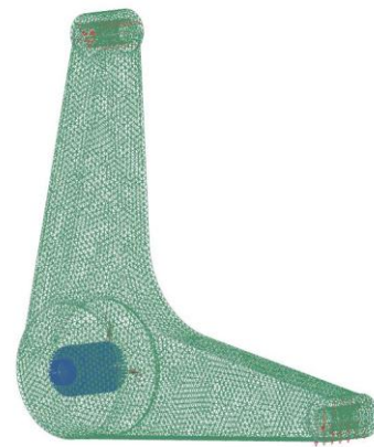
Figure 2. CAE data of primary product with loads and constraints
