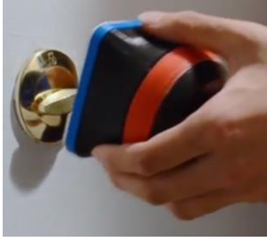
Figure 2. User-friendly installation requirements results in uncertain placement relative to the thumbturn's axis of rotation.
