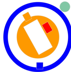
Figure 8. The accelerometer (red) should be on the end effector to keep track of the position of the thumbturn. The position of the transmission ring is not tracked directly, but its position can be deduced based on the history of motor commands and accelerometer values.
