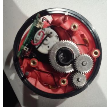
Figure 16. August has a complicated system of gears while requiring clearance for the accelerometer cable (hidden below other components), which results in its unusually large size compared to other smart locks.
