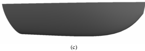
Fig. 11. 3D model hull with hull type variations: (a) Shallow Vee; (b) Deep Vee; and (c) Round Bottom.
