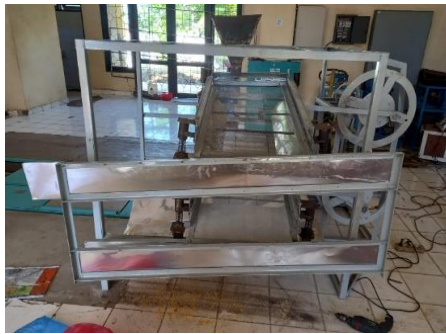
Fig. 7. The sifter machine with double filters for corn rice.
